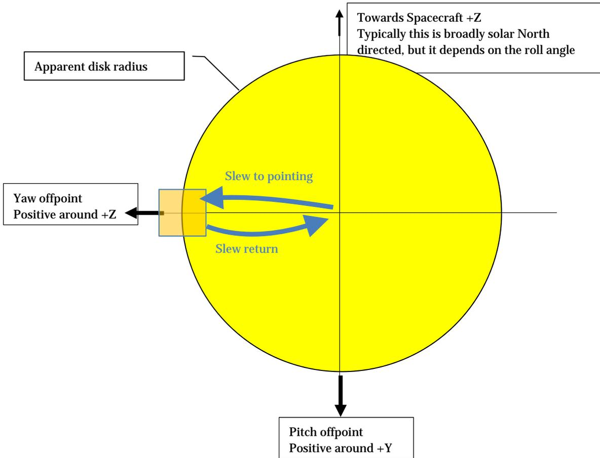
Figure 1, crude off-point diagram of out-of-field calibration if performed on the East limb
